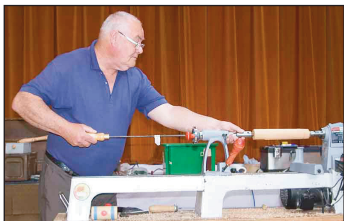
Having a go at long hole boring on the lathe.
