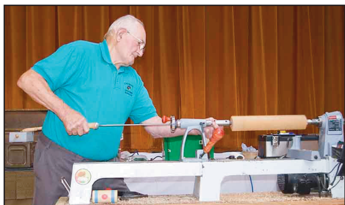
Having a go at long hole boring on the lathe.
