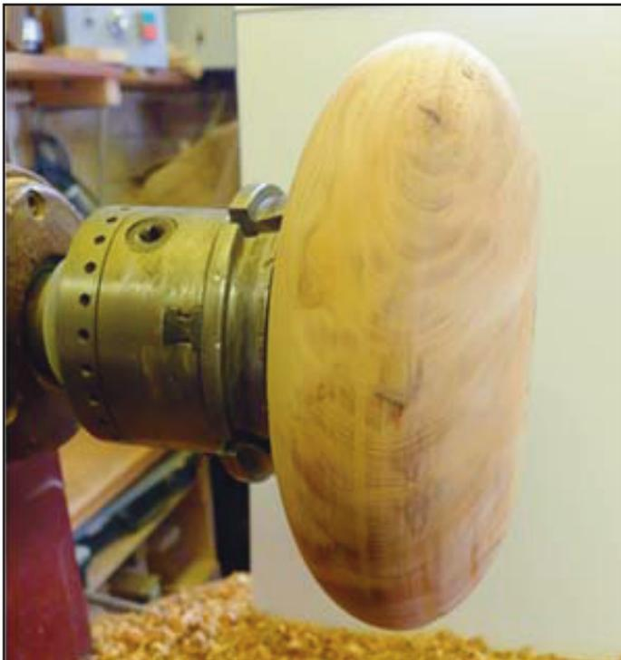
Now to the hollowing. This was completed with the Hamlet Little Brother. The Roly Munro tool and the Sorby scraper. The lathe
